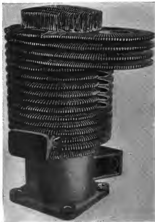
WIRE COILS RETAINED BY COPPER PLATING.
